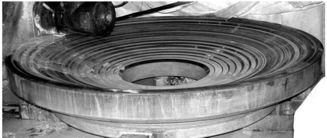
Figure 10: Machining of 2420 mm Hindle sphere ( $R_0 = 2510$  mm).
